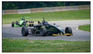
F2000 Championship Series drivers pilot fast and powerful open-wheel race cars at speeds of up to 145 m.p.h. With a two-liter Ford or Mazda powerplant, the cars weigh around 1,200 lbs and utilize Hoosier tires. Paired with aerodynamics, the race cars generate downforce, allowing them faster turning speeds.
